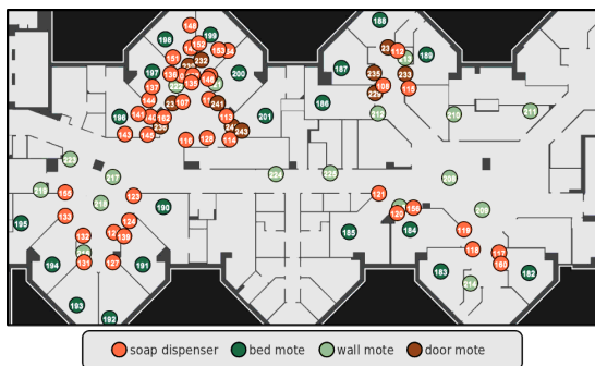
Figure 2: Placement of the stationary sensors or beacons in the Medical Intensive Care Unit.
